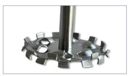
In the laboratory, dispersion of dry wax can be achieved with a disk tip speed of 1,000 – 1,500 feet per minute (FPM), or around 5 – 7 meters per second (m/s). In a production environment, a tip speed of 4,000 – 5,000 FPM, or around 22 – 26 m/s, is a good target.
